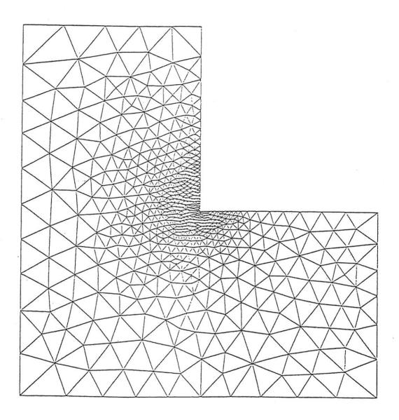
Fig.3: Adaptive triangulated mesh
