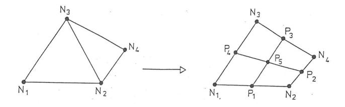
Fig.4: Quadrilaterals created by splitting of two neighboring triangles
