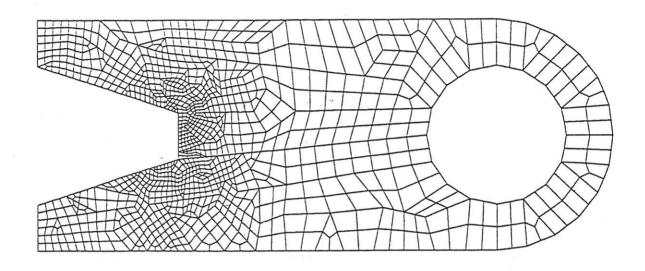
Fig.6: Refined quadrilateral mesh ( no relaxation )
