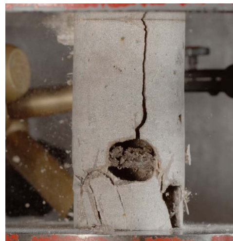
Fig. 1: Picture of the fracturing specimen taken with the high-speed camera.
